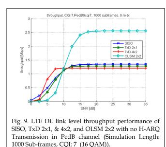
In this simulation, the CQI value is set to 7, the 16 QAM is used as the modulation scheme and the maximum number of HARO re-transmissions to zero.
