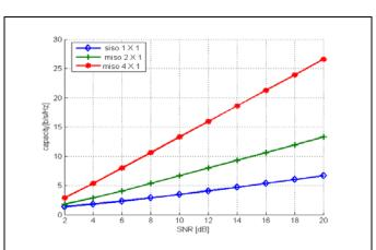
Fig. 6. Capacity of SISO and MISO compared. As can be seen in figure 6, the MIMO system achieved higher capacity at the expense of SNR which is undesirable in mobile communication capacity.
