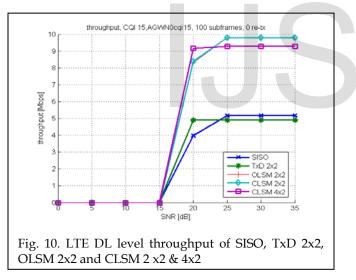
The maximum throughput in MIMO scheme depends on number of transmit antennas and the number of data streams (layers). In the case of OLSM, two spatially separated data streams are transmitted thus leading to twice the maximum throughput of the 4x2 TxD system. Note that the results in figure 8 were obtained with channel adaptive pre-coding. The throughput results are shown in figures 10 and 11.
